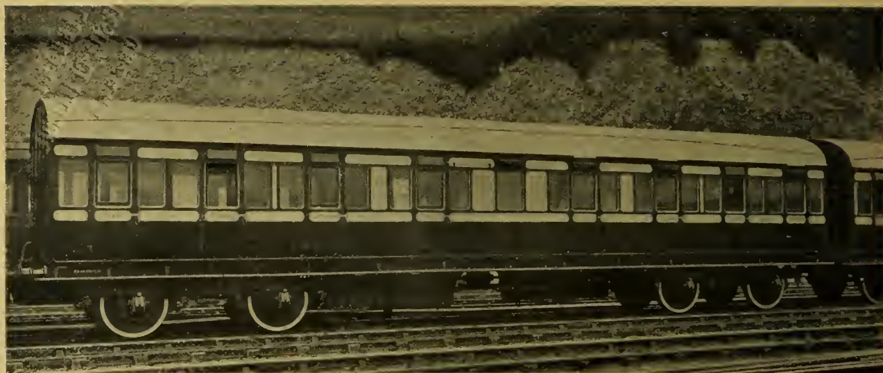
COMPOSITE COACH DESIGNED BY MR. D. EARLE MARSH, LOCO., CARRIAGE & WAGON SUPT., L. B. & S. C. RY., LENGTH 54-FT., WIDTH 8-FT. 6-IN.
