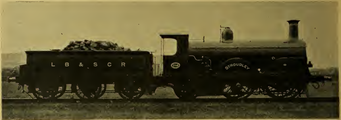
FRONT-COUPLED EXPRESS PASSENGER LOCOMOTIVE No. 184, NOW RE-NAMED "STROUDLEY," LONDON, BRIGHTON & SOUTH COAST RY.
