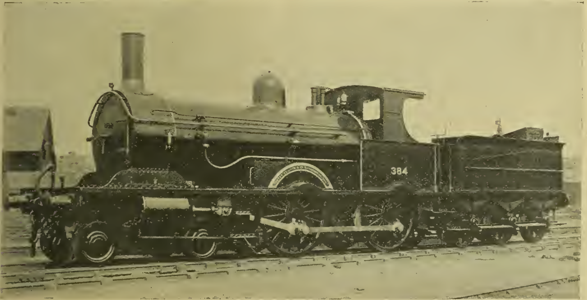
FIG. 54.—FOUR WHEELS COUPLED BOGIE MIXED TRAFFIC LOCOMOTIVE NO. 384, LONDON & SOUTH WESTERN RY.
