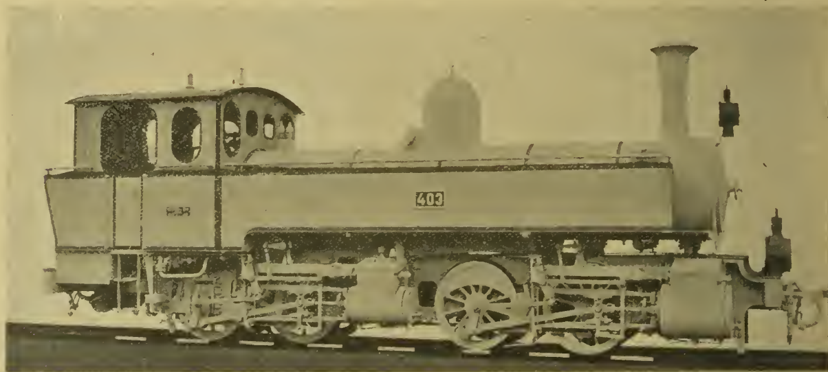
MEYER FOUR-CYLINDER COMPOUND LOCOMOTIVE No. 403, PORTUGUESE STATE RYS.
