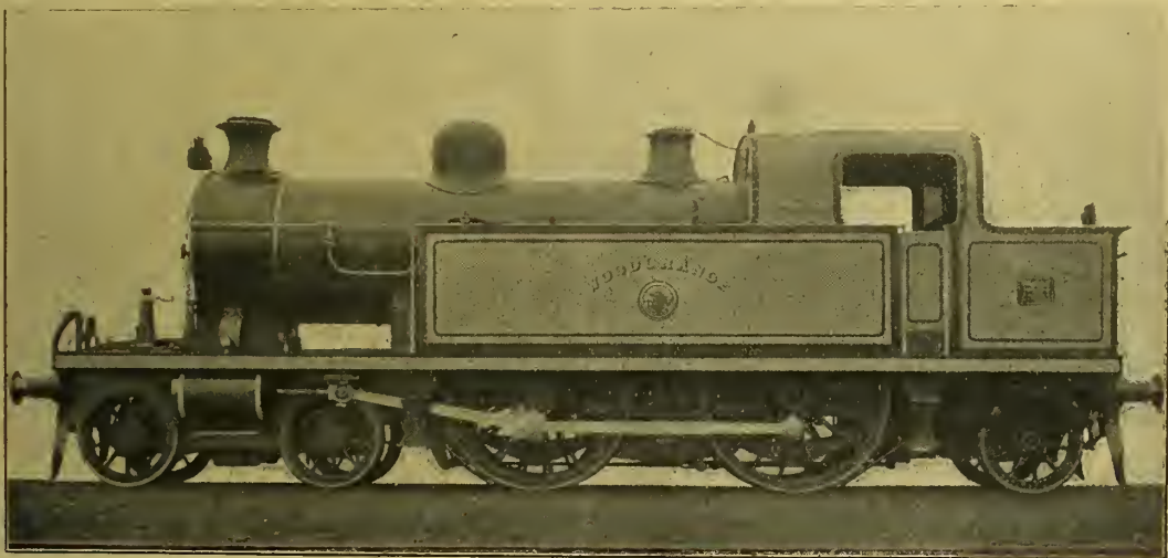
REBUILT FOUR-COUPLED BOGIE PASSENGER TANK LOCOMOTIVE No. 37 "WOODGRANGE," LONDON, TILBURY & SOUTHEND RY.
