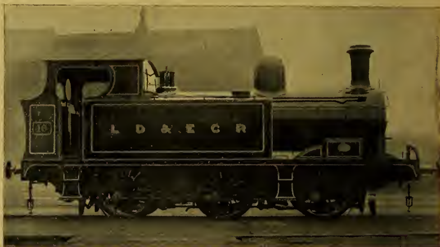
Photo by SIX-COUPLED TANK LOCOMOTIVE No. 10, CLASS B, L. D. & E. C. RY. Loco. Pub. Co. Ltd.
