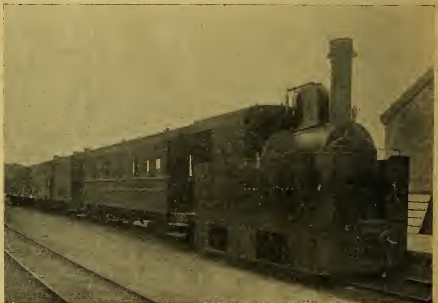
FOUR-COUPLED TANK LOCOMOTIVE No. 2, REBUILT, SCHULL & SKIBBEREEN LIGHT RY.
