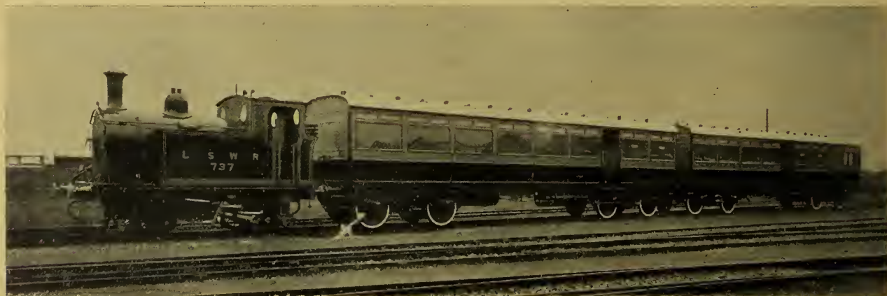
STEAM RAIL MOTOR, INTERMEDIATE COACH AND TRAILER, LONDON & SOUTH WESTERN RY.
