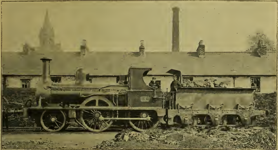
FOUR-WHEELS COUPLED PASSENGER LOCOMOTIVE NO. 4, NORTHERN COUNTIES COMMITTEE, MIDLAND RY.
