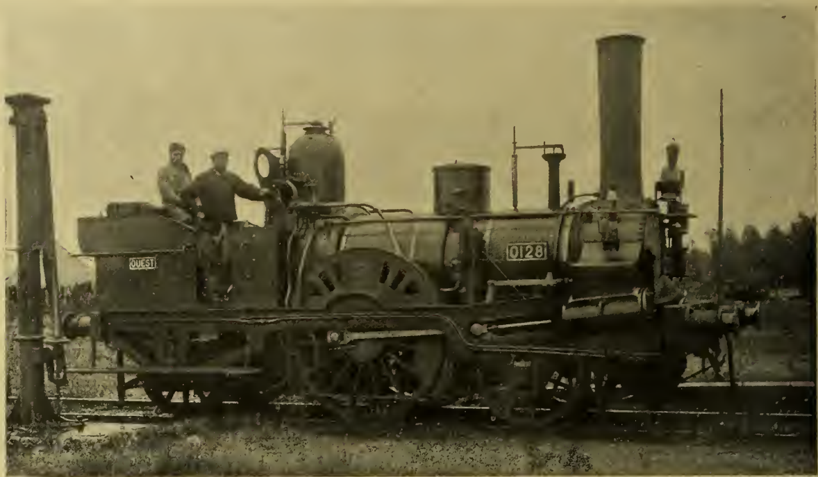
SINGLE DRIVER TANK LOCOMOTIVE No. 0128, WESTERN RY. OF FRANCE.
