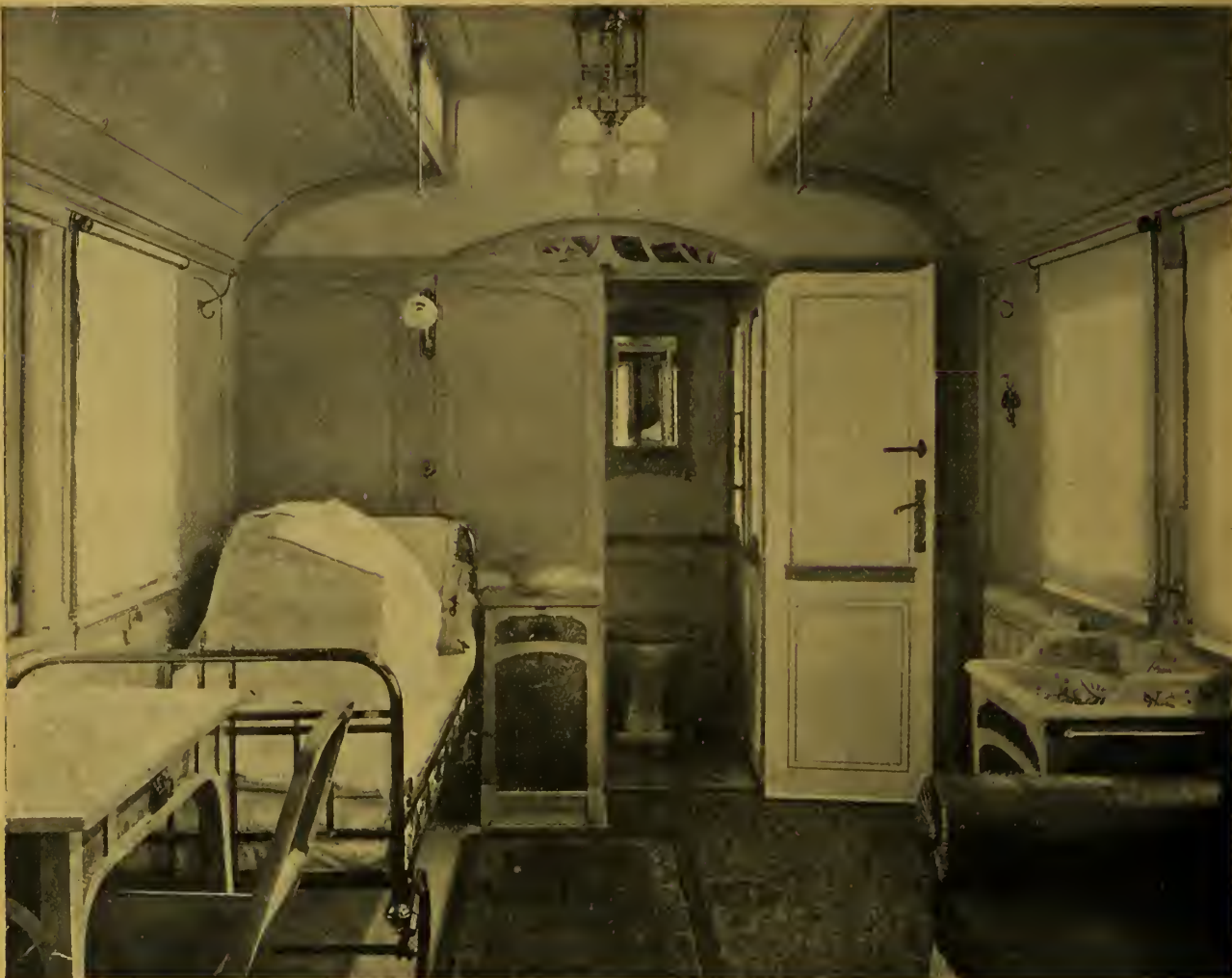
Interior of Invalid's Carriage, Hungarian State Rys. —This is a most completely fitted vehicle, specially designed for the transport of invalids and their attendants. This view shows the invalid's room, but there are in addition a completely equipped dispensary, and a compartment for the traveller's attendants.
