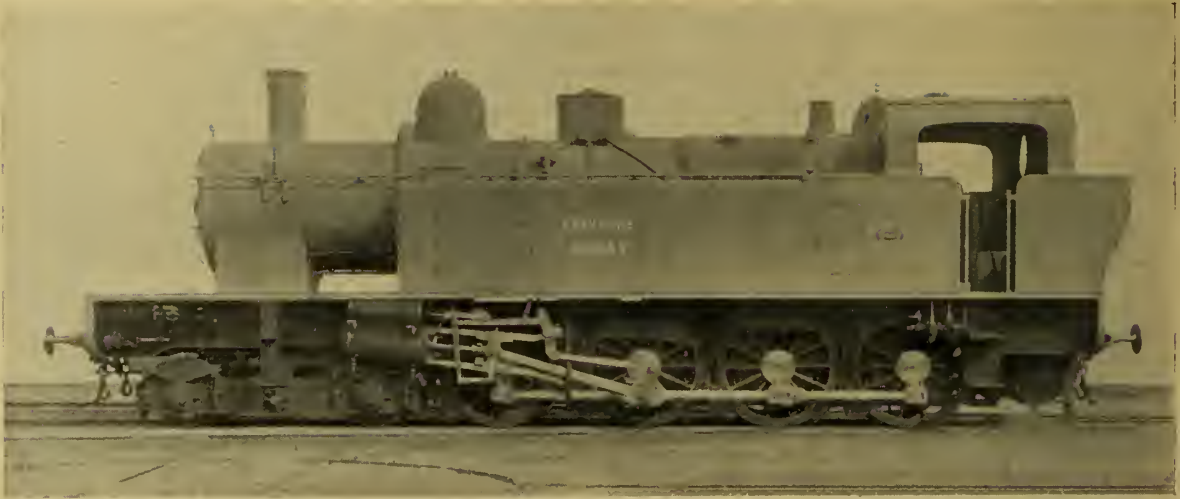
EIGHT WHEELS COUPLED BOGIE FOUR-CYLINDER COMPOUND TANK LOCOMOTIVE NO. 4005, CEINTURE RY., PARIS.
