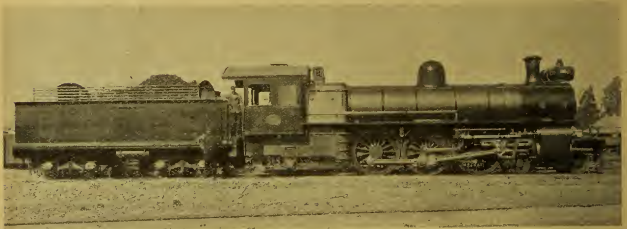
No. 650, 4-6-2 LOCOMOTIVE, 10TH CLASS, CENTRAL SOUTH AFRICAN RYS.
