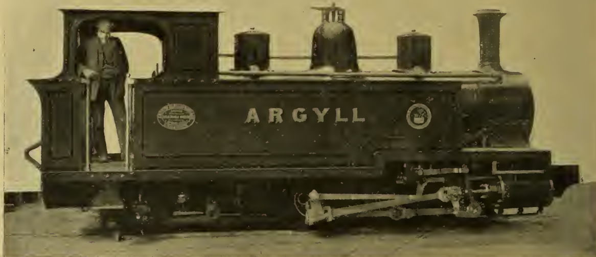
SIX-COUPLED TRAILING RADIAL TANK LOCOMOTIVE "ARGYLL," CAMPBELTOWN & MACHRIHANISH LIGHT RY.
