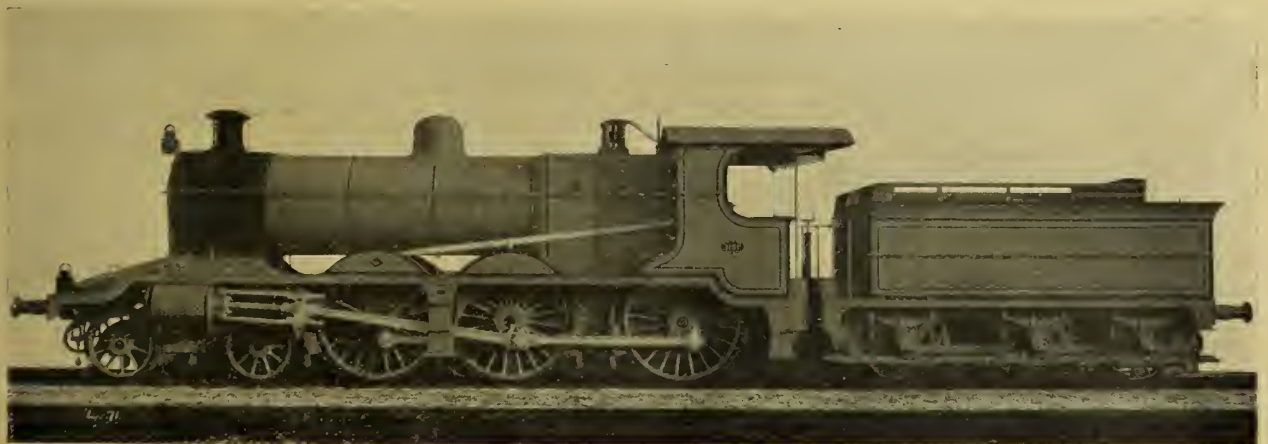
SIX-COUPLED BOGIE EXPRESS PASSENGER LOCOMOTIVE, EAST INDIAN RY.
