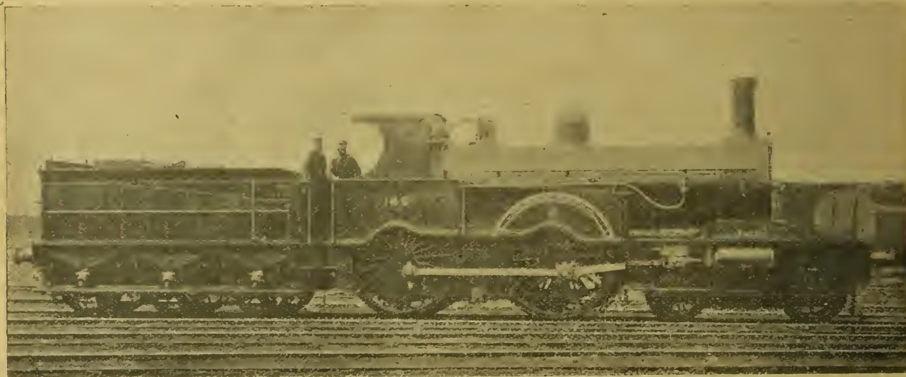
FIG. 55.—FOUR WHEELS COUPLED BOGIE EXPRESS PASSENGER LOCOMOTIVE No. 146, LONDON & SOUTH WESTERN RY.
