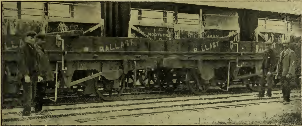
FIG. 1.—RAIL LOADER IN FIRST POSITION WITH RAIL LIFTED ON TO SUPPORTS.
