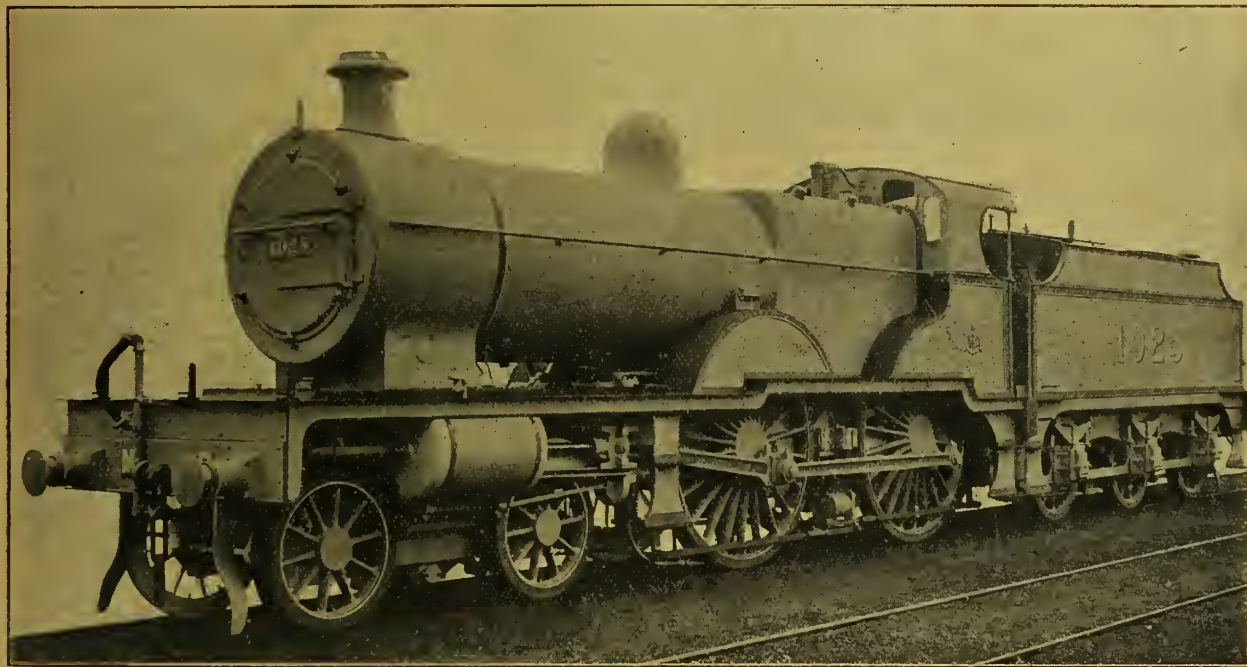
THREE-CYLINDER COMPOUND EXPRESS LOCOMOTIVE No. 1025, MIDLAND RY.
