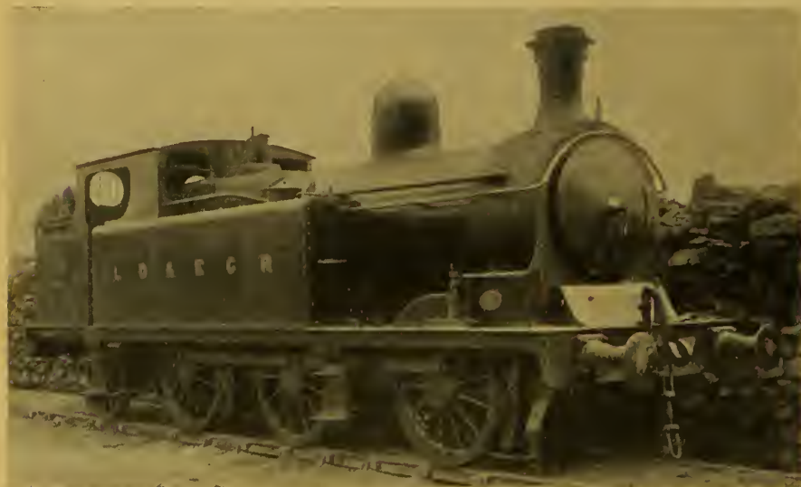
Photo by SIX-COUPLED RADIAL TANK No. 7, CLASS A, REBUILT, L. D. & E. C. RY. Loco. Pub. Co. Ltd.
