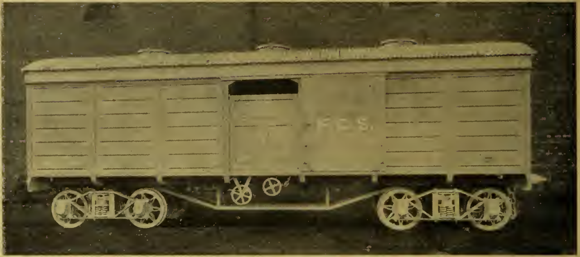
4-TONS COVERED GOODS WAGON, BUENOS AYRES GREAT SOUTHERN RY. (Particulars on preceding page.)
