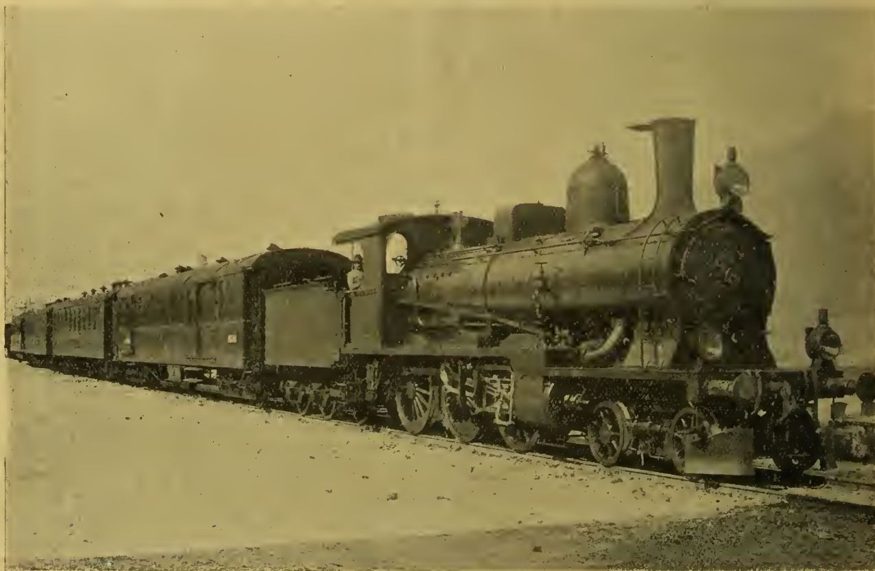
SIX-COUPLED BOGIE LOCOMOTIVE No. 228, AND TRAIN OF NEW CARRIAGE STOCK, GOTHARD RY.
