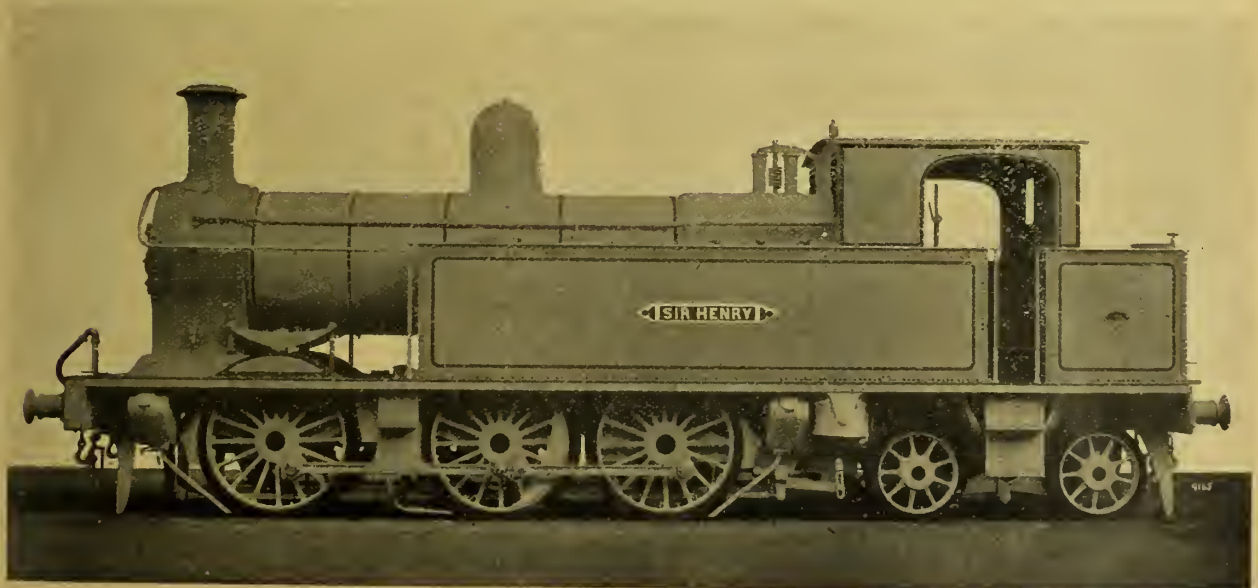
SIX-COUPLED TRAILING BOGIE TANK LOCOMOTIVE "SIR HENRY," SLIGO, LEITRIM & NORTHERN COUNTIES RY.
