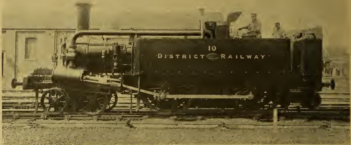
STANDARD COUPLED BOGIE PASSENGER LOCOMOTIVE No. 10 (REBUILT), METROPOLITAN DISTRICT RY.
