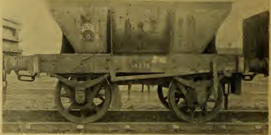
6-TONS MINERAL WAGON, NORTH BRITISH RY.
