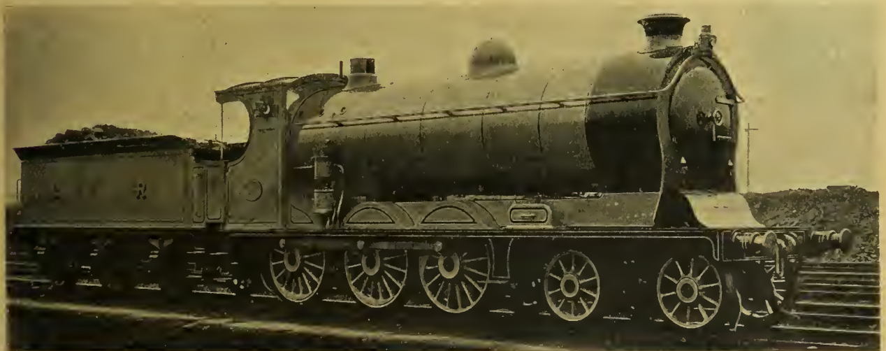
SIX-COUPLED BOGIE GOODS LOCOMOTIVE No. 918, CALEDONIAN RY.
