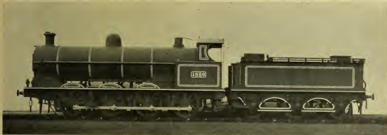
THREE-CYLINDER COMPOUND COAL ENGINE No. 1866, REBUILT AS TWO-CYLINDER SIMPLE ENGINE, LONDON & NORTH WESTERN RY.
