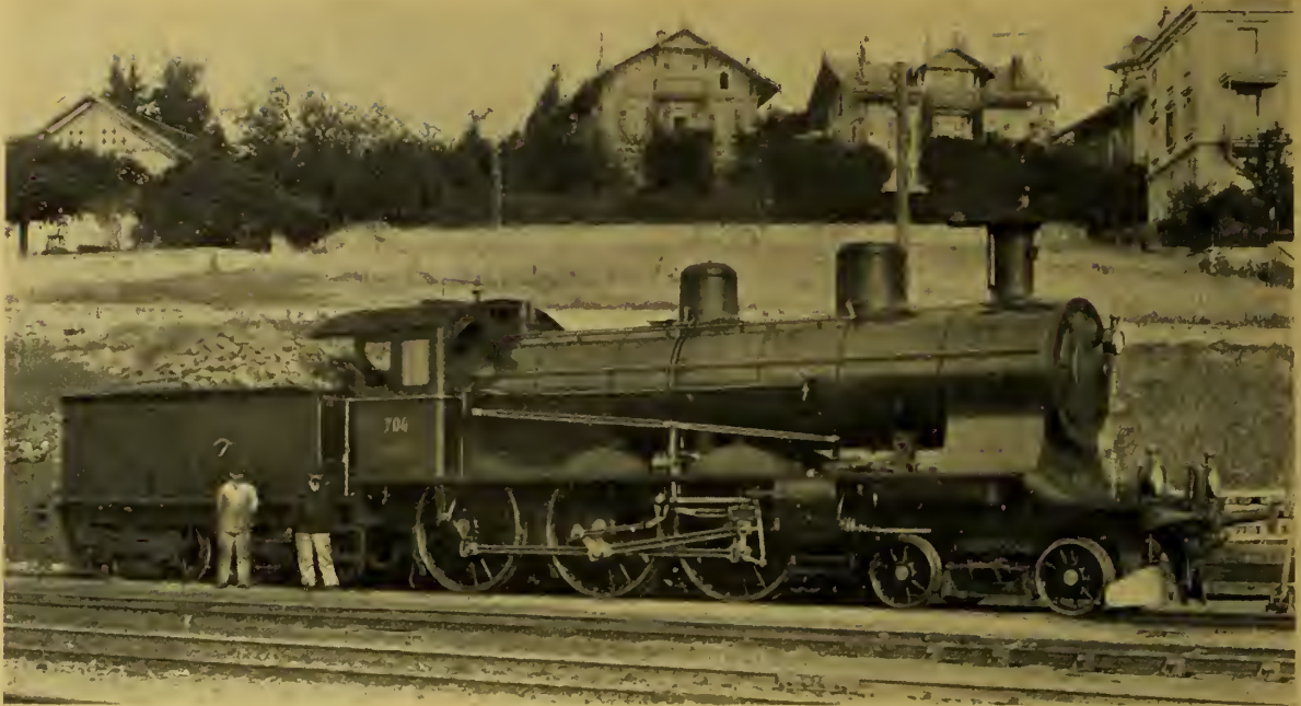
TEN-WHEEL FOUR-CYLINDER COMPOUND PASSENGER LOCOMOTIVE No. 704, CLASS A 3 3/4 , SWISS STATE RYS.
