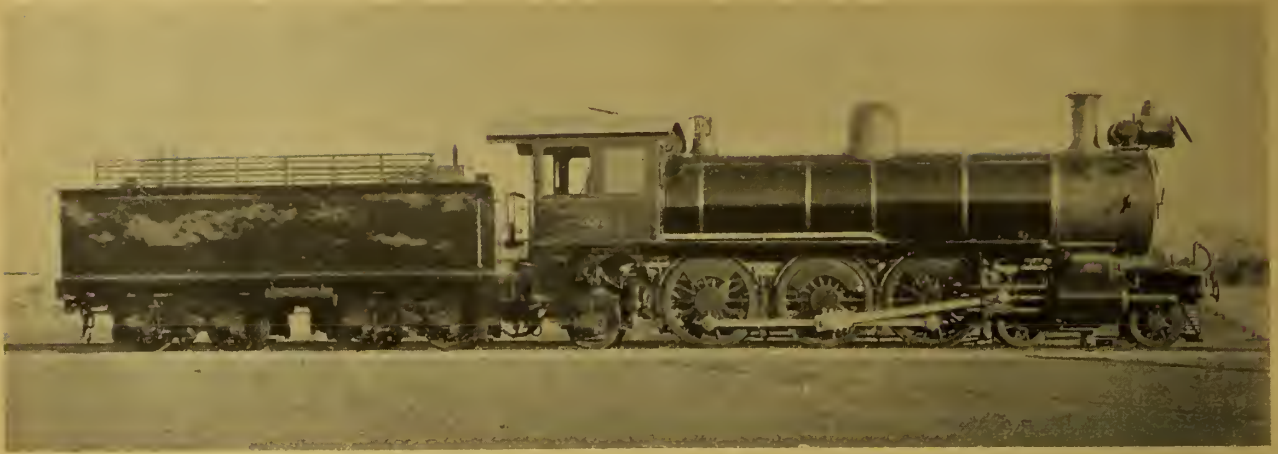
No. 603, 4-6-2 LOCOMOTIVE, 9TH CLASS, CENTRAL SOUTH AFRICAN RYS.
