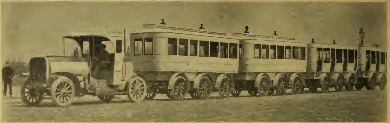
RENARD PETROL MOTOR ROAD PASSENGER TRAIN FOR SERVICE IN HUNGARY.
