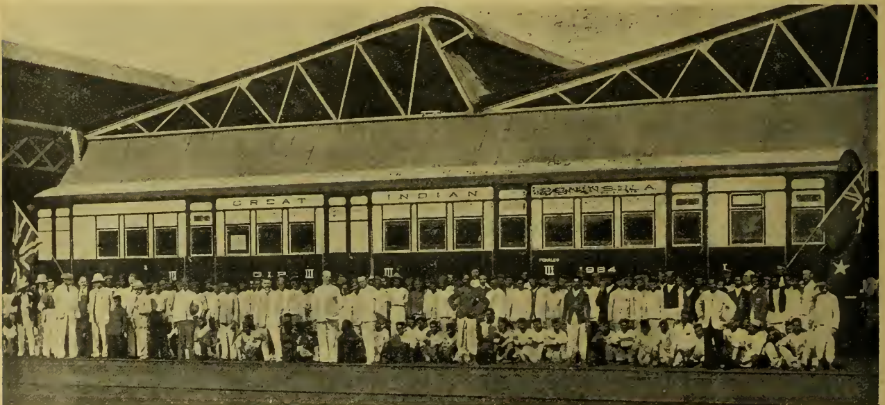
TRAILER CAR FOR COMBINED STEAM RAIL MOTOR TRAIN, BUILT IN 10 HOURS, GREAT INDIAN PENINSULA RY.
