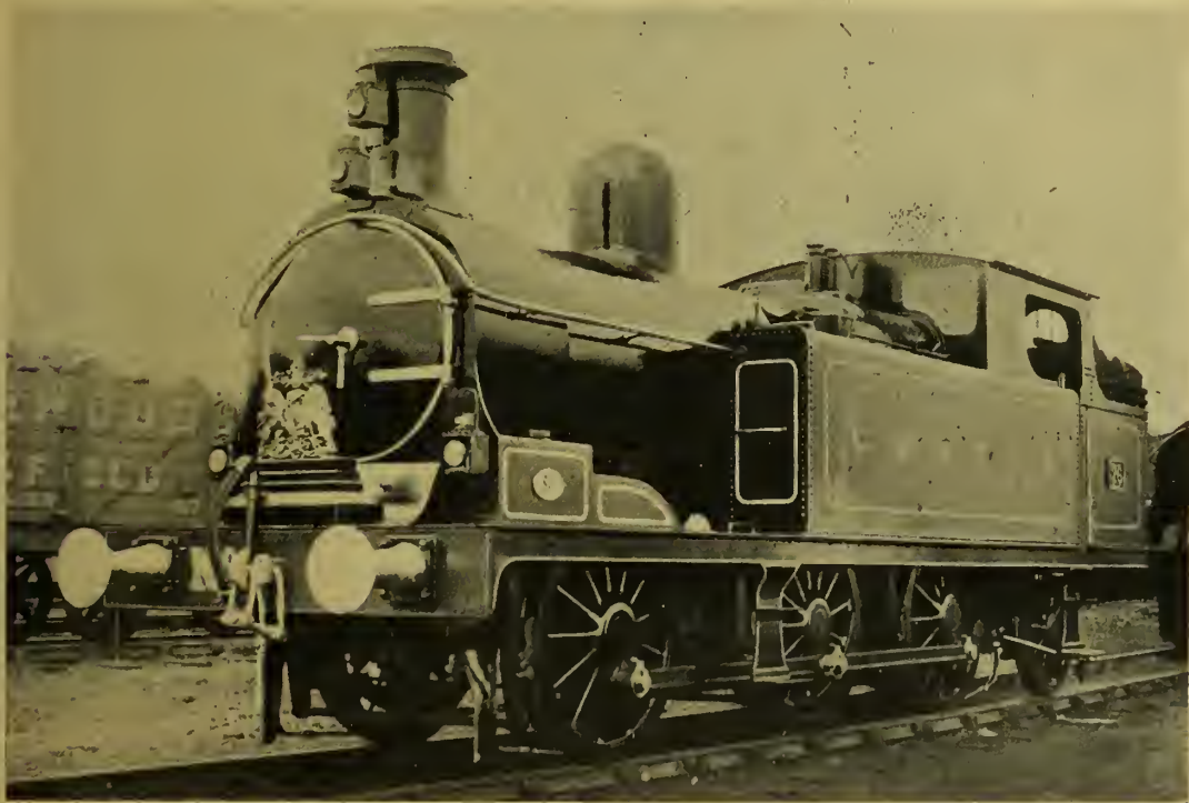
SIX-COUPLED RADIAL TANK LOCOMOTIVE No. 26, CLASS A, WITH MARSHALL'S VALVE GEAR, L. D. & E. C. RY.
